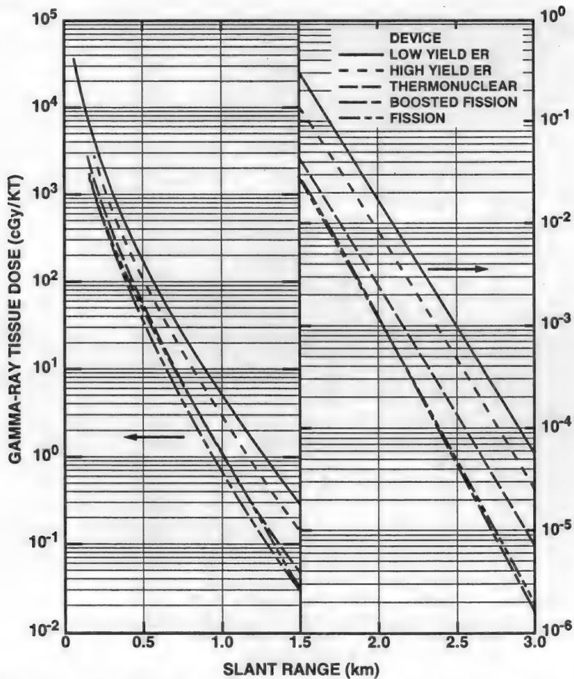
Figure 8.27. Total Gamma-Ray Dose per Kiloton Yield Versus Slant Range From Neutron Activation of European Soil for Various Nuclear Weapon Types.
